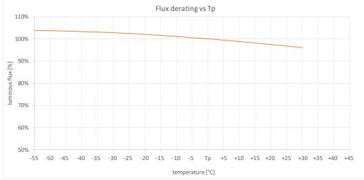
Note: Light flux varies with the temperature measured @Tc point; nominal values is given @Tc = Tp. Flux increases when Tc decreases.
